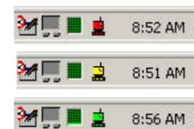
You should now see a small icon for the Configuration Utility in the system tray by your clock. The Configuration Utility is used to change or verify the configuration information that relates to your 22 Mbps Wireless PC Card or PCI Adapter. The Configuration Utility icon will be colored to indicate the status of your wireless network: red for disconnected, yellow for connected with poor quality, and green for connected with good quality.
