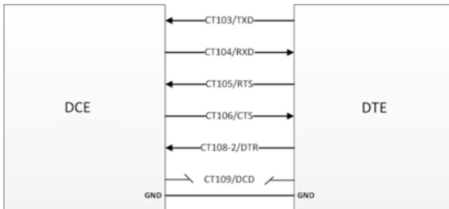
Figure 16. V24 Serial Link Implementation for a 5-wire UART
