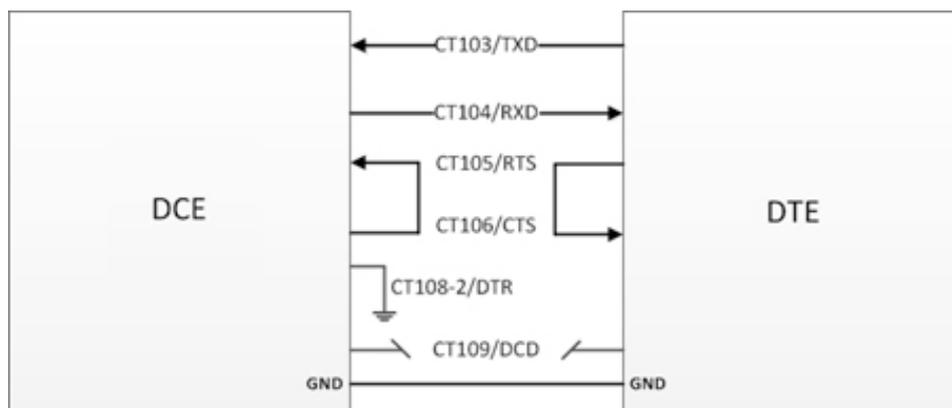
Figure 18. V24 Serial Link Implementation for a 2-wire UART
