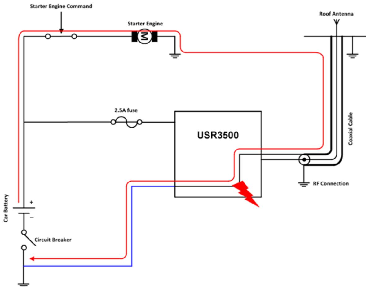
Figure 28. Example of an Electrical Connection That May Damage the modem
