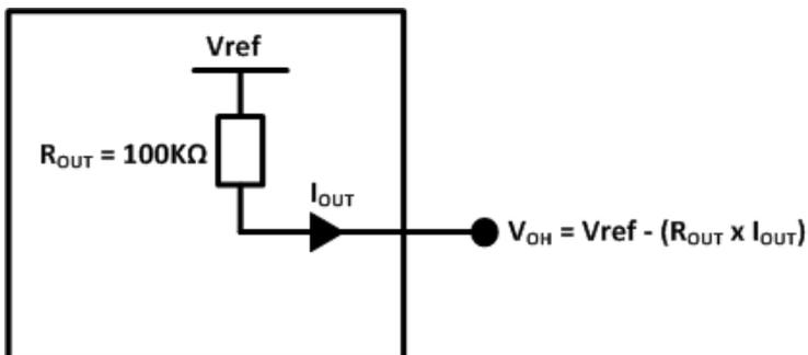
Figure 13. Equivalent circuit of  $V_{OH}$ ,  $V_{ref} > 2.8V$
