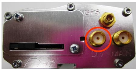
Figure 23. Secondary RF Connector for USR3500
