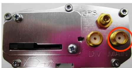
Figure 22. Main RF Connector
