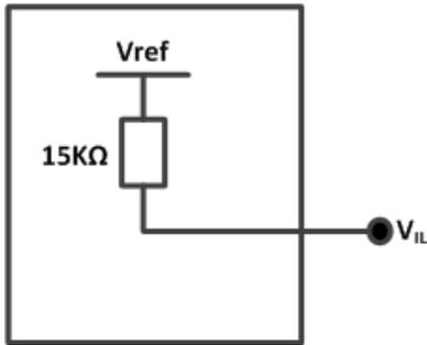
Figure 10. Equivalent Circuit of  $V_{IL}$ ,  $V_{ref} > 2.8V$
