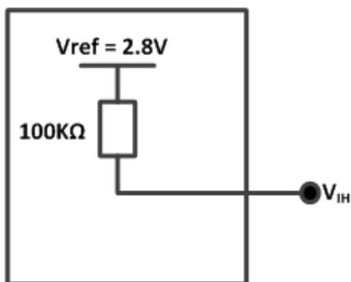
Figure 7. Equivalent Circuit of  $V_{IH}$ ,  $V_{ref} = 2.8V$
