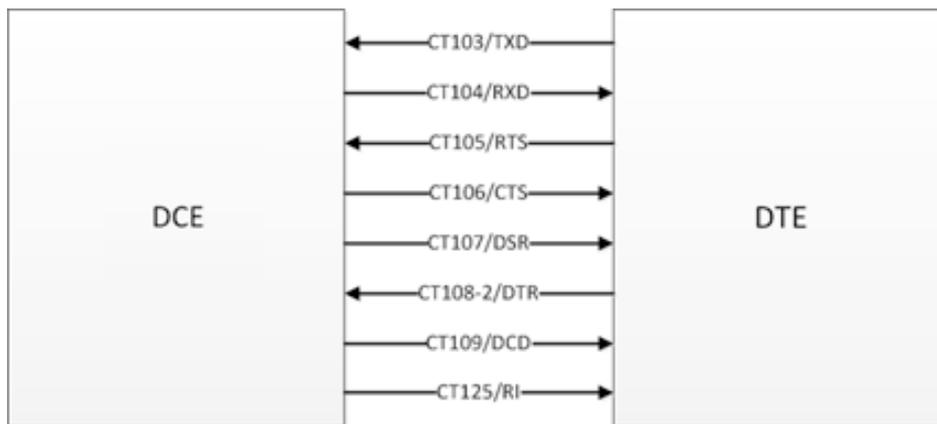
Figure 15. RS232 Serial Link Signals
