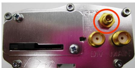
Figure 24. GPS RF Connector for USR3500
