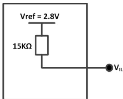
Figure 6. Equivalent Circuit of  $V_{IL}$ ,  $V_{ref} = 2.8V$
