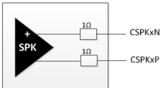
Figure 19. Equivalent Circuit of CSPK
