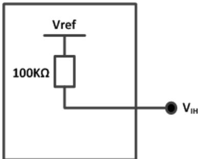
Figure 11. Equivalent circuit of  $V_{IH}$ ,  $V_{ref} > 2.8V$
