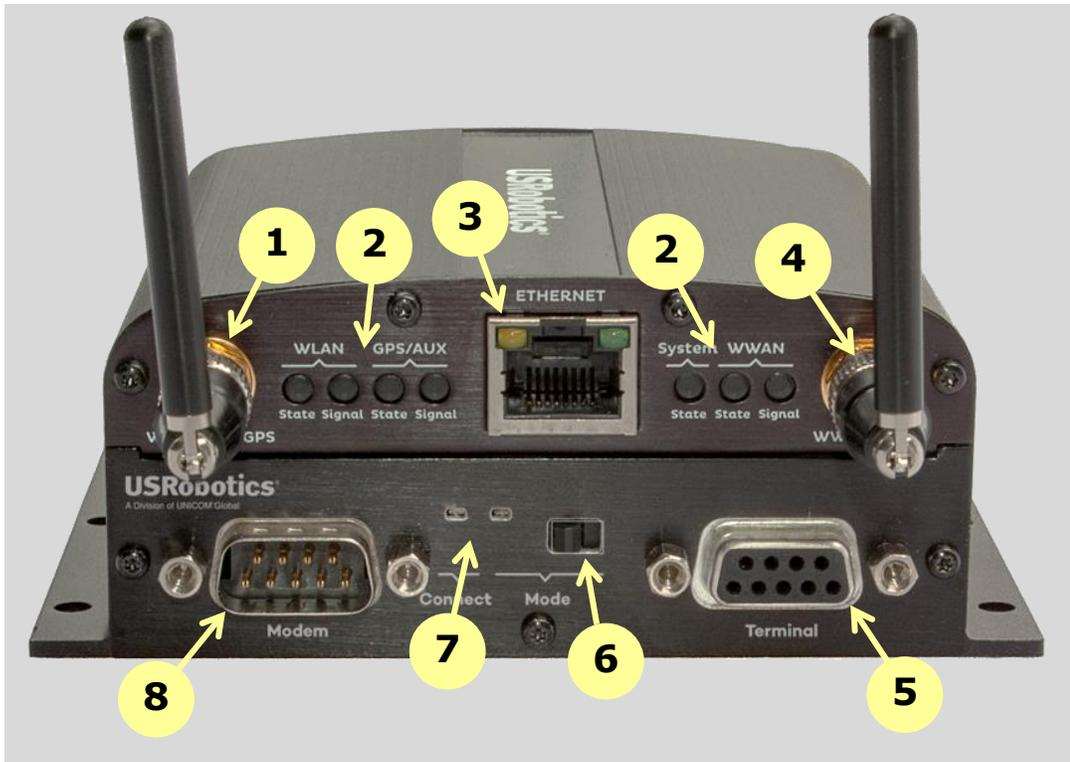
1. **WWAN Diversity Antenna Connector** - SMA-female antenna port for connection to a diversity antenna or a GPS antenna. See the [USR3520/USR803520 Gateway User Guide](#) for details.
