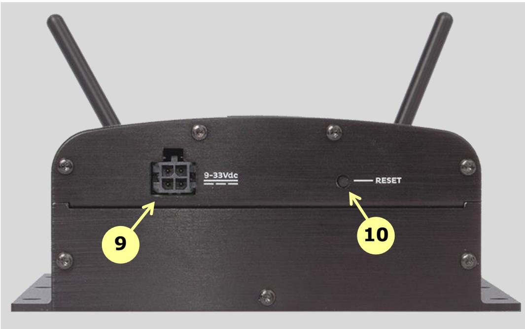
**9. External Power Supply Input** – This input receives operating power from the external low voltage power supply that is included with the base unit. Connect the included power supply to this connector. See the [USR3520/USR803520 Gateway User Guide](#) for details.
