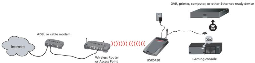
Ad Hoc (sometimes referred to as peer-to-peer), is a type of wireless network allowing a wireless adapter or other Ethernet-ready device to connect directly to another wireless adapter or Ethernet-ready device. The graphic below depicts one example of an ad hoc network.
