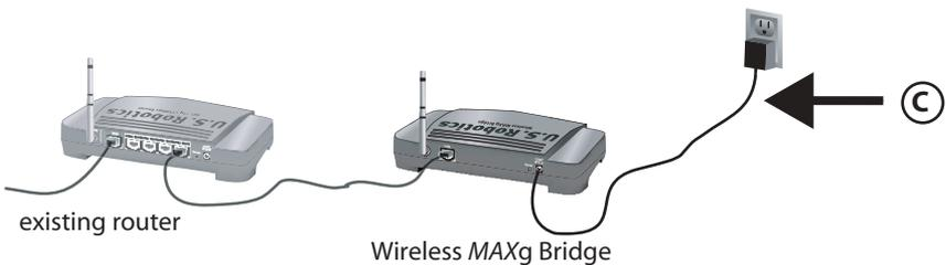
**Note to UK Users:** Attach the correct power plug to the power adapter.
