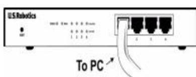
Connect one end of an Ethernet cable to your PC's Ethernet adapter. Connect the other end to one of the LAN ports on the Broadband Router.
