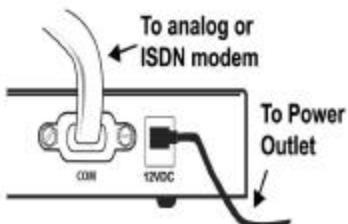
Connect the included power cord to the power jack on the Broadband Router. Plug the power cord into a standard power outlet. The Broadband Router will automatically enter the self-test phase. Turn on your PC and your analogue or ISDN modem.
