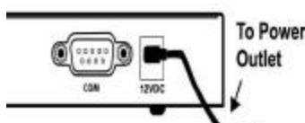
Turn on your Cable or DSL modem. Connect the included power cord to the power jack on the Broadband Router. Plug the power cord into a standard power outlet. The Broadband Router will automatically enter the self-test phase. After the self-test phase is complete, turn on your PC.
