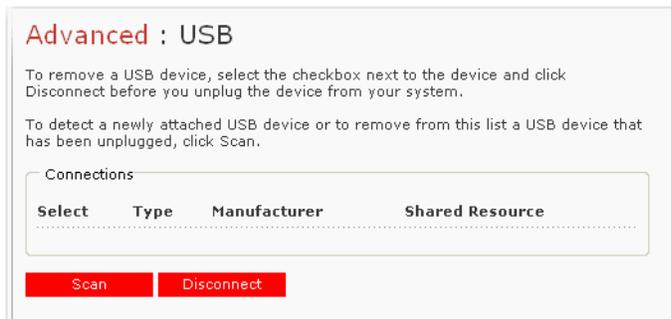
When you plug a USB device into the storage system, the storage system automatically detects it and adds that device to the **USB** page. (You might need to click **Scan** to update the display.)
