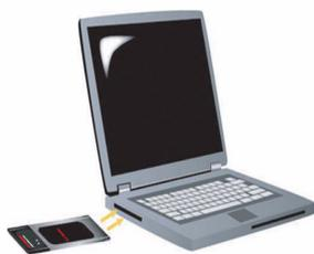
Locate an available PC Card slot and fully insert the 22 Mbps Wireless PC Card. PC Card slots are typically on the side of laptops. You should hear a beep when the 22 Mbps Wireless PC Card is fully inserted and detected.
