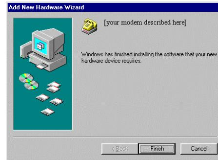
6. When Windows is finished copying files, you should verify that the modem installation was a success. Click the Windows **Start** button and point to **Settings**. Then click **Control Panel**.
