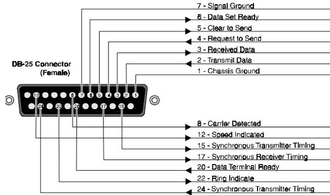
**Wiring a DB-25 to DB-9 Cable**
