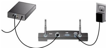
The Wireless Access Point has three LED status indicators: PWR, TX/RX, and WARN. When the Wireless Access Point is plugged in, the PWR LED will be illuminated. When a network connection is established, the TX/RX LED will be illuminated. If an unauthorized user attempts to use the 802.11g Wireless Turbo Multi-function Access Point, the WARN LED will be illuminated.
