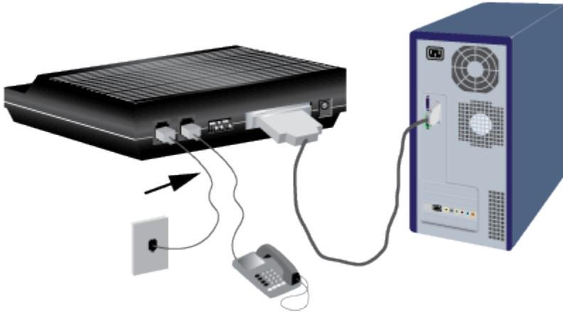
3. To connect a telephone through the modem, plug the telephone's cord into the modem's
