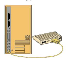
Connect the power adapter to your modem and plug it into the wall.
