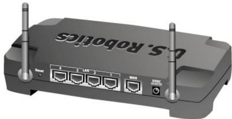
**RESET Button:** Press in and hold the RESET button for between five and ten seconds. This will reset the Wireless Turbo Access Point & Router to the factory default settings.
